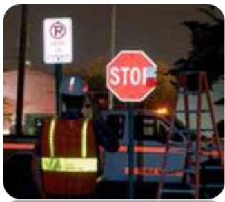
Shown above is a technician measuring the retroreflectivity of a stop sign.
