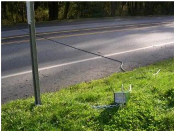
Traffic counts are taken by placing a rubber hose across the road. When a vehicle crosses the hose, an air pulse is sent to an automatic traffic recorder. Sometimes dual rubber hoses are used to determine vehicle classification (such as commercial vehicles) and to measure the speed of vehicles.
