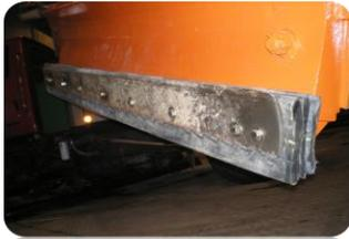
*Shown above is a rubber tire that has been cut and installed on a wing plow blade.*
