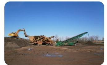
The above picture shows the topsoil screening process in action at the North Holland garage. The Road Commission rents a topsoil screening machine as needed.
